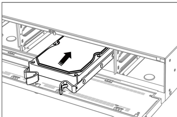
**Figure 1-6 Insert HDD**
