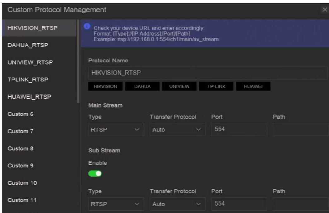
Figure 6-3 Add Network Camera via Customized Protocol
