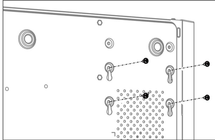
**Figure 1-11 Fix HDD to Device Bottom**
