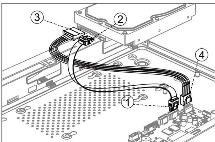
Figure 1-10 Connect Cables
