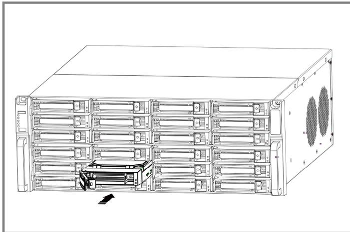
**Figure 1-8 Push HDD Case into Slot**
