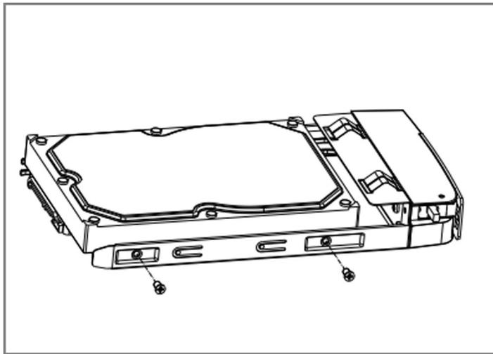
**Figure 1-7 Fix HDD**
