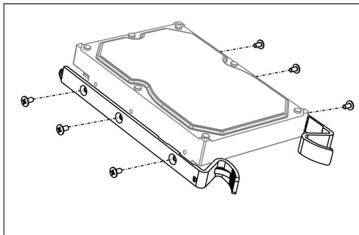
**Figure 1-4 Fix Mounting Ears to HDD**
